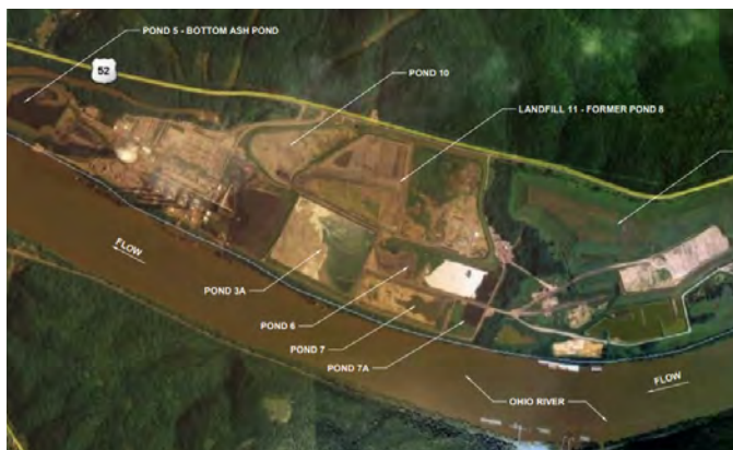
EPA-labeled aerial imagery of the J.M. Stuart coal plant on the Ohio River. Only one of the five coal ash ponds assessed was in “satisfactory” condition. 61 Image: EPA
